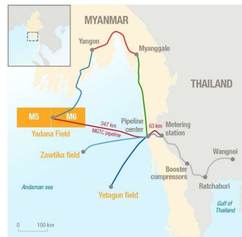
Exhibit 11: Yadana project location
