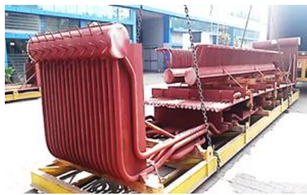
Exhibit 28: Water wall panels
